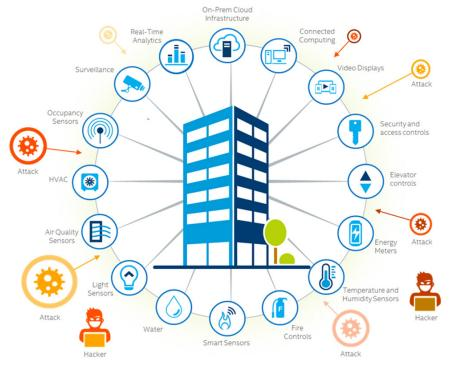
Buildings are becoming more intelligent through the connection of many different systems, including BACs, BMSs, access controls, environmental, and IoT networks, as shown in the diagram above. This growing connectivity can create critical security exposures capable of generating occupant safety, financial, and reputational risks.
